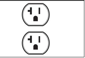
Use each receptacle to operate 120 Volt AC, single-phase, 60 Hz electrical loads requiring up to 2,400 watts (2.4 kW) at 20 Amps of current. Use cord sets that are rated for 125 Volt AC loads at 20 Amps (or greater).
